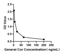
The standard curves are provided for demonstration only. A standard curve should be generated for each set of Cor assayed.
